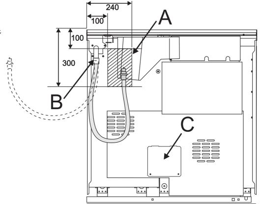
Although a 900mm hose can be used, a 1250mm hose will allow slightly more flexibility in the positioning of the bayonet and make moving the cooker easier. The hose should be fitted so that both inlet and outlet connections are vertical so that the hose hangs downwards.
